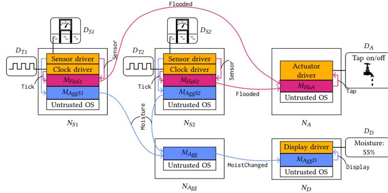
Fig. 2. Our running example with two applications,  $A_{Agg}$  (blue) and  $A_{Flo}$  (red). Hardware ( $N_*$  and  $D_*$ ) is trusted; the OS and the network are untrusted. E.g., the  $A_{Flo}$  deployer creates the three red Software Modules (SMs) (cf. Fig. 3a) with a trusted compiler, attests the shared sensor-, clock- and display drivers and sets-up connections between the SMs. Remote attestation assures authentic execution of  $A_{Agg}$  and  $A_{Flo}$ .
