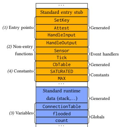
Fig. 8. Memory layout of the compiled version of module  $M_{FloS1}$  in application  $A_{Flo}$  (Fig. 3a). The code- and data sections are shaded in yellow and blue, respectively. The numbers on the left labels correspond to the compiler inputs, while the right labels indicate whether parts are implicitly generated by the compiler or correspond to source code.
